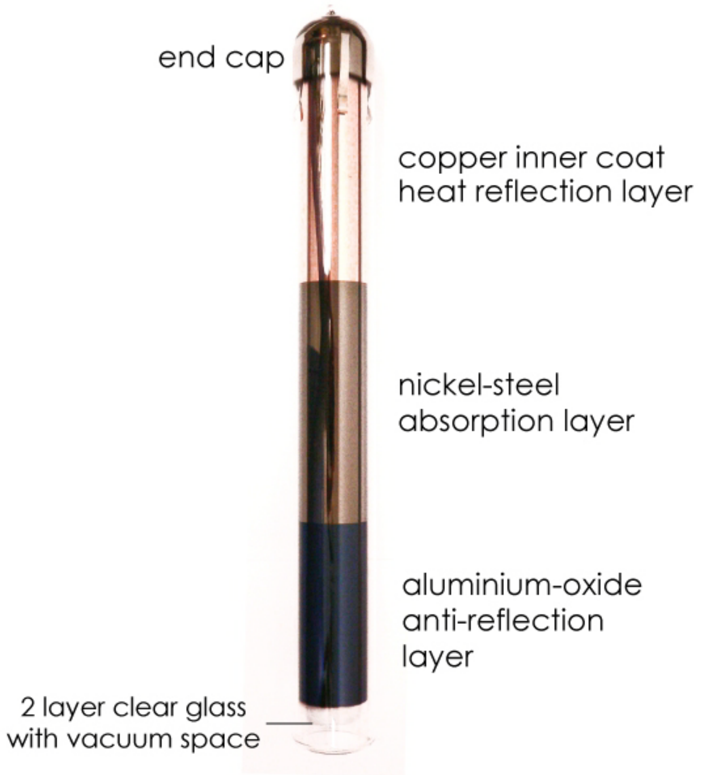
Cut-away-view of 3-traget vacuum tube showing each layer.
